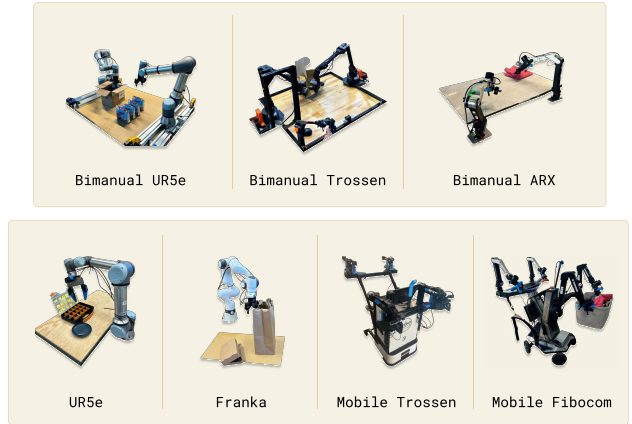
Fig. 5: The robots used in our experiments. These include single and dual-arm manipulators with 6-DoF and 7-DoF arms, as well as holonomic and nonholonomic mobile manipulators. \pi_0 is trained jointly on all of these platforms.
