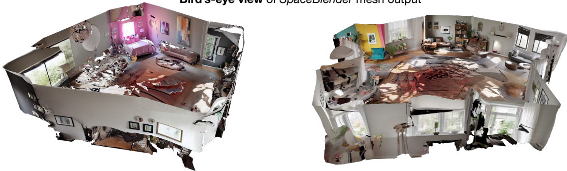
Figure A.4: Examples of spaces generated with various numbers of submeshes. Left: a SPACEBLENDER mesh based on four input images, all featuring corners. Right: a SPACEBLENDER mesh based on five input images featuring a mixture of room shapes.
