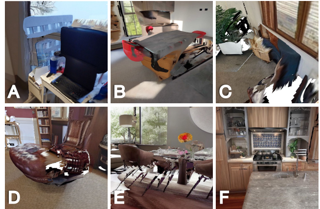
Figure 12: Examples of SPACEBLENDER pipeline components errors: (A) protrusion of outdoor structure, (B) distorted table, (C) depth estimation error, (D) depth alignment error, (E) depth estimation error, (F) floor expansion error.
