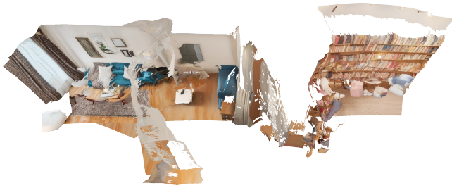
Figure 2: A birds-eye view of two meshes that failed to blend due to the lack of geometric guidance and context throughout the iterative mesh completion process.
